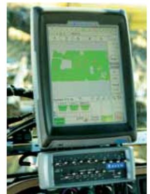
The Raven Viper Pro field computer allows farmers to control multiple seeding functions on one display screen, helping eliminate in-cab clutter.
