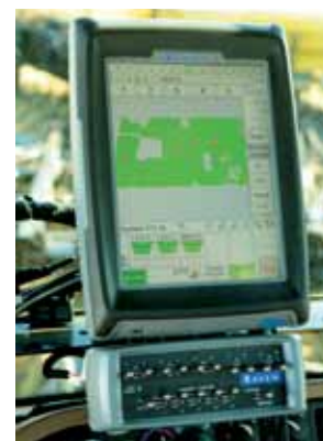
The Raven Viper Pro field computer allows farmers to control multiple seeding functions on one display screen, helping eliminate in-cab clutter.
