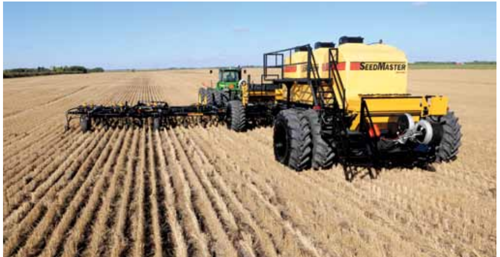
The Nova XP-820 Smart Cart proved it can handle more than 400 lbs/acre of fertilizer with absolutely no plugging on the SeedMaster Research Farm this fall.
